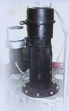
US Navy Warping Winch Drive
