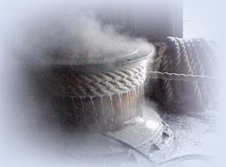
US Navy Warping Winch Drive
