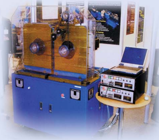
Show Equipment: Belt Test Stand
