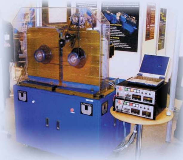
Show Equipment: Belt Test Stand
