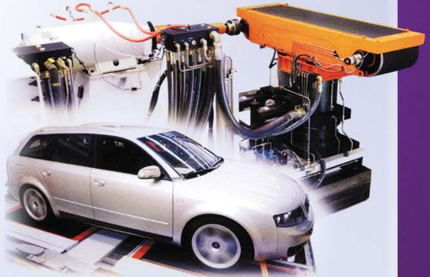
Photo courtesy of "MTS Systems" MTS Flat-Trac® Dynamic Roadway enables repeatable ride evaluation combining vertical inputs and an active drive train.
